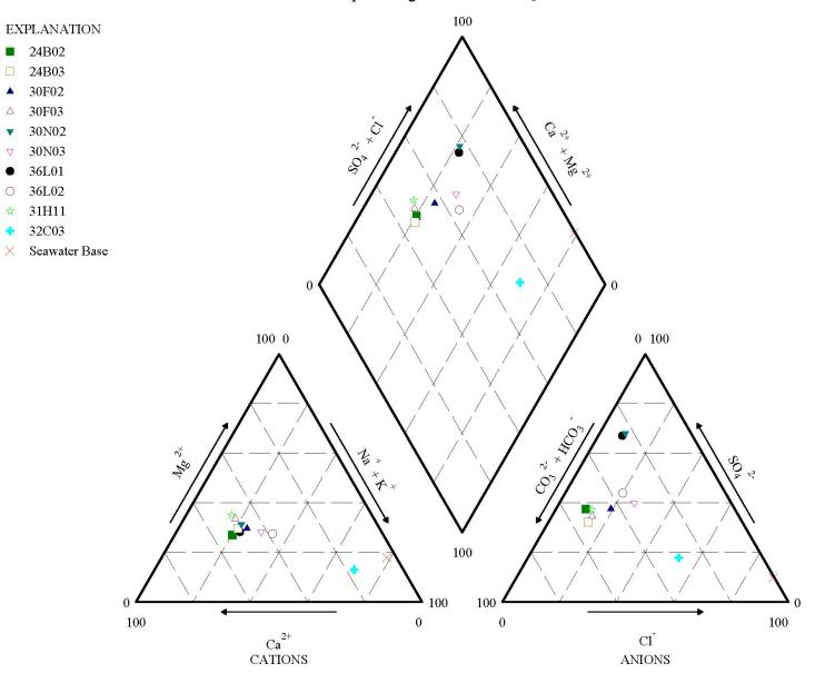
FIGURE 23A. PIPER DIAGRAMS OF WATER QUALITY IN SELECT MONITORING WELLS - 2023 Q1 RESULTS Northern Cities Management Area San Luis Obispo County, California
