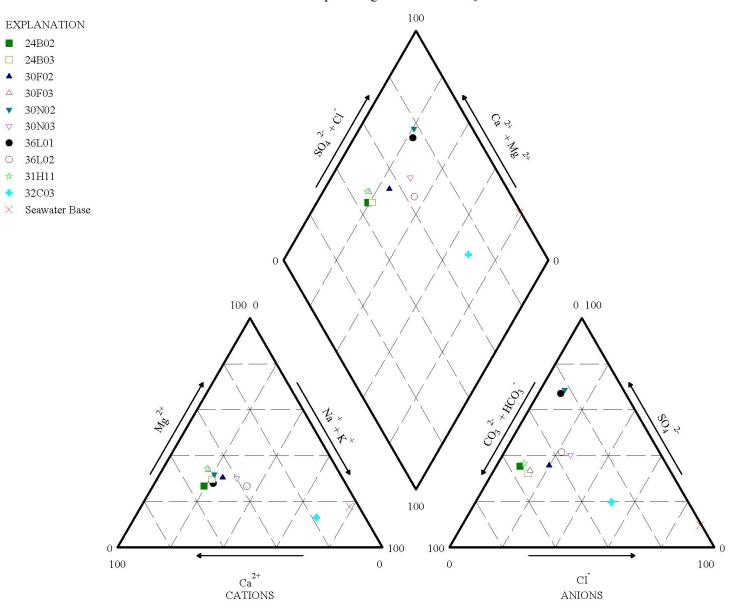
FIGURE 23D. PIPER DIAGRAMS OF WATER QUALITY IN SELECT MONITORING WELLS - 2023 Q4 RESULTS Northern Cities Management Area San Luis Obispo County, California
