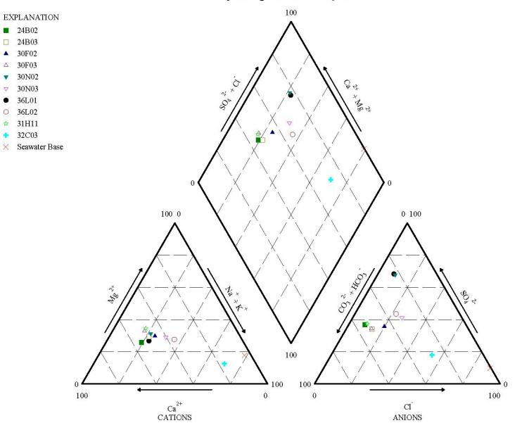
FIGURE 23C. PIPER DIAGRAMS OF WATER QUALITY IN SELECT MONITORING WELLS - 2023 Q3 RESULTS Northern Cities Management Area San Luis Obispo County, California
